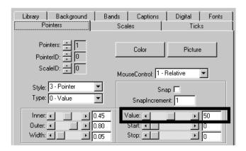
The **Value** property indicates the current pointer value. Set the initial value to 0, halfway between the maximum and minimum scale values. Click **OK** to accept the changes and close the dialog box.
