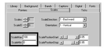
To modify the scale range, change **ScaleMax** to 20 and **ScaleMin** to -20.
