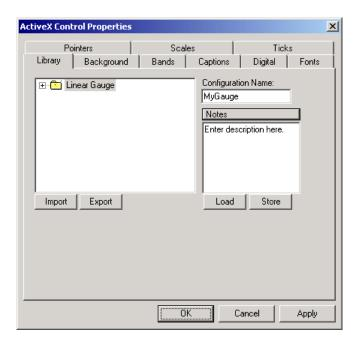
An alternative to this procedure is to export customized controls to .gms files. To do this, select a directory from the left side of the panel and click **Export**. You can later access these controls by using the **Import** button, or share the controls by sharing the .gms files.
