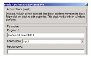
• The block is driven by a customized S-function, ax\_pie\_sfun.m, rather than the S-function that drives the original library block. To see this, select the outer border of the block and choose **Edit** -> **Look under mask** from the model window's menu.
