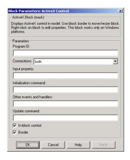
**Note** Double-clicking the border of a preconfigured block (supplied with the blockset) displays its ActiveX Control Properties dialog box, which lists properties in multiple tabbed panels. Double-clicking a block that you created by customizing the generic ActiveX Control block displays its Block Parameters dialog box.
